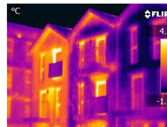
An image of the difference in heat loss between identical homes, but the end house has yet to have cavity wall insulation installed (source: Jez Wingfield, UCL Energy Institute).
